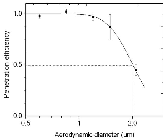
FIG. 3. The penetration of the cyclone as a function of particle size.
