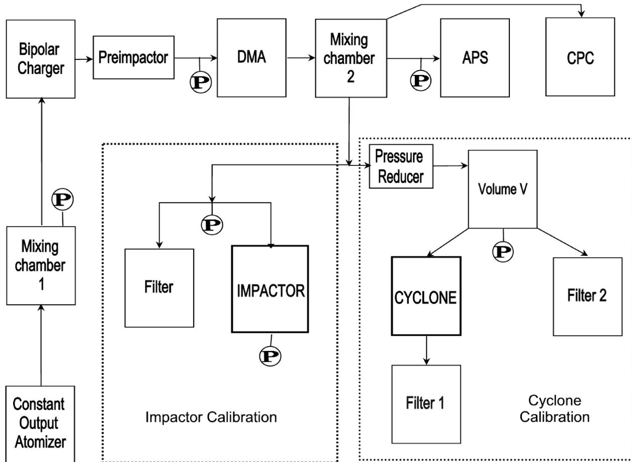
FIG. 2. The setup used in determining of the penetration of the cyclone arrangement and the setup used to determine the collection efficiency of the aerosol sampler.
