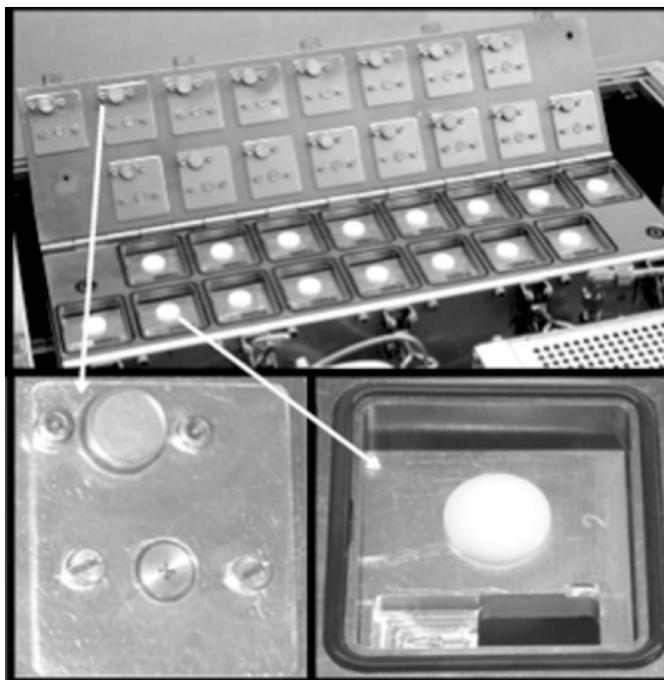
FIG. 1. The aerosol sampler, with the lid in its open position, consisting of 16 channels. Details are showing the nozzles (left) and the position where the samples are placed (right).
