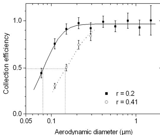
FIG. 4. The collection efficiency of the aerosol sampler as a function of particle size.
