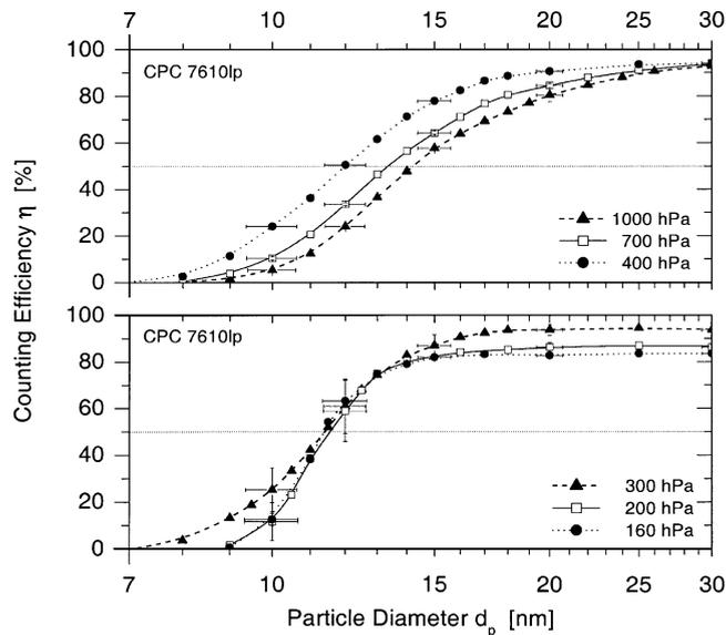
Fig. 2. CPC 7610lp counting efficiency at 160, 200, 300, 400, 700 and 1000 hPa. Error bars (not given for each point) indicate one standard deviation of the DMA transfer window ( $x$ -axis) and the standard deviation of the counting efficiency mean value ( $y$ -axis).
