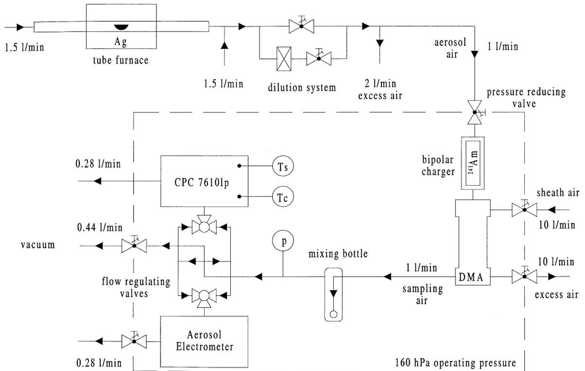
Fig. 1. Low-pressure calibration set-up. The sign “*p*” denotes a piezoelectric pressure gauge, “*T<sub>s</sub>*” the saturator temperature sensor, and “*T<sub>c</sub>*” the condenser temperature sensor. Downstream the pressure reducing valve, the set-up is operated at lower pressures down to 160 hPa. Volume flow rates are given at laboratory pressure and temperature.
