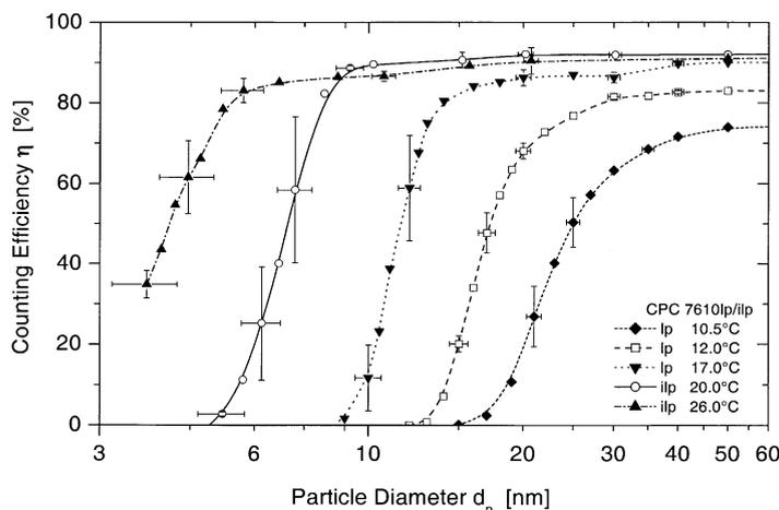
Fig. 5. Counting efficiency curves of the CPC 7610lp and CPC 7610ilp for 10.5, 12, 17, 20, and 26°C temperature difference. Operating pressure is 200 hPa. Measurements were performed with either NaCl particles (10.5°C) or Ag particles (other curves).
