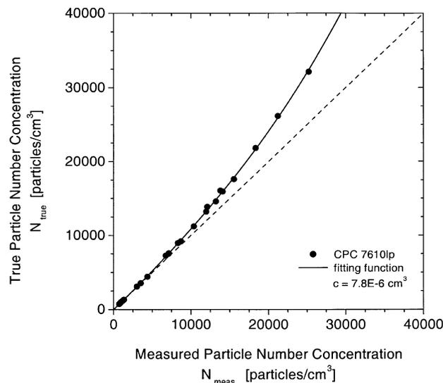
Fig. 9. Particle coincidence curve for the CPC 7610lp. The solid line shows a fitting function to the measurement points according to Eq. (2). The dotted curve indicates the one to one line. “ $c$ ” gives the coincidence parameter defined in Eq. (1).
