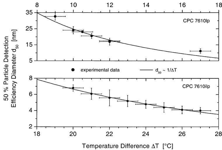
Fig. 6. Fifty percent particle detection efficiency diameter  $d_{50}$  of the CPC 7610ilp and CPC 7610lp as function of temperature difference  $\Delta T$ . The solid line denotes the relation  $d_{50} \sim 1/\Delta T$ . Measurements were performed at 200 hPa operating pressure. Error bars indicate the experimental uncertainty of the temperature measurement ( $x$ -axis) and the standard deviation of the mean  $d_{50}$  values ( $y$ -axis).
