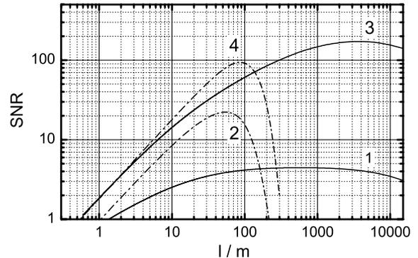
Fig. 2. Calculated SNR. OA-ICOS, solid lines 1 (PDA400) and 3 (PDA10DT) for  $\overline{P_0} = 20 \text{ mW}$ , single-pass absorption  $A(\nu_0) = 1 \times 10^{-5}$ ,  $L = 0.3 \text{ m}$ ,  $T_M = 1$ ,  $C_P = 1$ . TDLAS, dashed lines 2 (PDA400) and 4 (PDA10DT) for  $R = 0.99$ .
