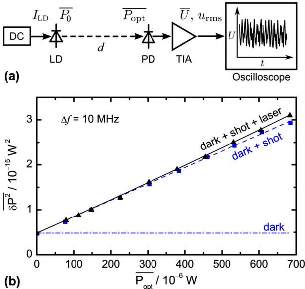
Fig. 1. (Color online) (a) Constant injection current,  $I_{\text{LD}}$ , is provided to the LD.  $\overline{P_{\text{opt}}}$  is detected by a PD. Mean voltage  $\overline{U}$  and fluctuation  $u_{\text{rms}}$  are measured by an oscilloscope at the output of a TIA. (b) Variance of noise power ( $\overline{\delta P^2}$ ) as a function of mean optical power ( $\overline{P_{\text{opt}}}$ ) showing dark noise, shot noise, and laser excess noise contributions.
